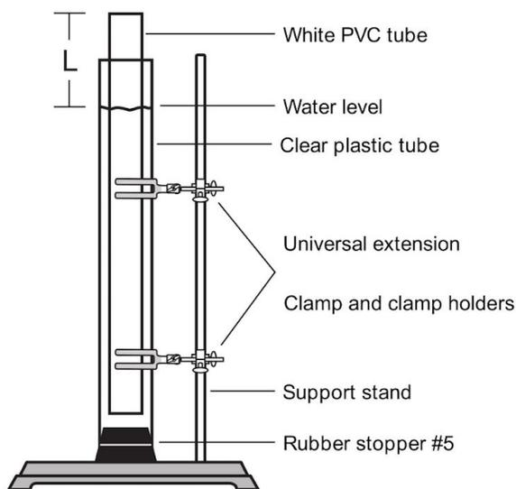
4. Place the white PVC tube inside of the clear plastic tube.
